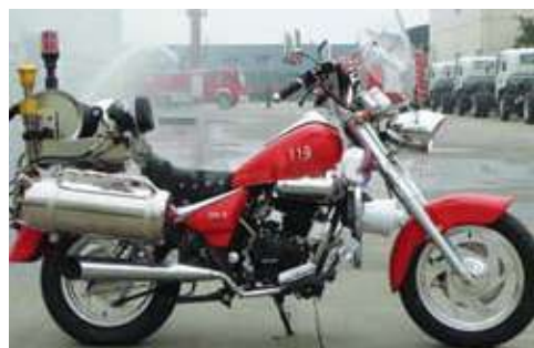
Big Motor cycle with back pack mist fire fighting unit
