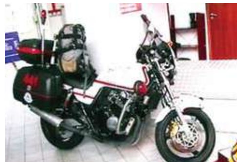
Small Motor Cycle water mist fire fighting unit
