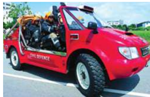
Small vehicle with 500 litres capacity water mist fire fighting unit
