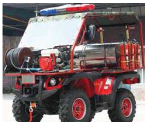
Small 500 liters water mist fire fighting vehicle
